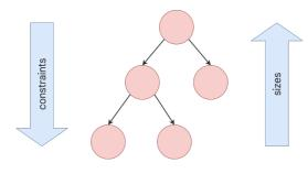
To perform layout, Flutter walks the render tree in a depth-first traversal and passes down size constraints from parent to child. In determining its size, the child must respect the constraints given to it by its parent. Children respond by passing up a
