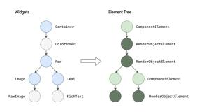
In the build phase, Flutter takes the widget tree and translates it into a corresponding *element tree*, with one element per widget.
